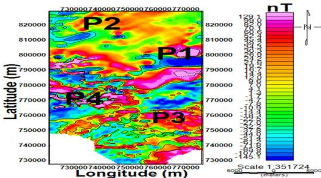
**Figure 8:** Residual magnetic contour grid map showing four profiles.
