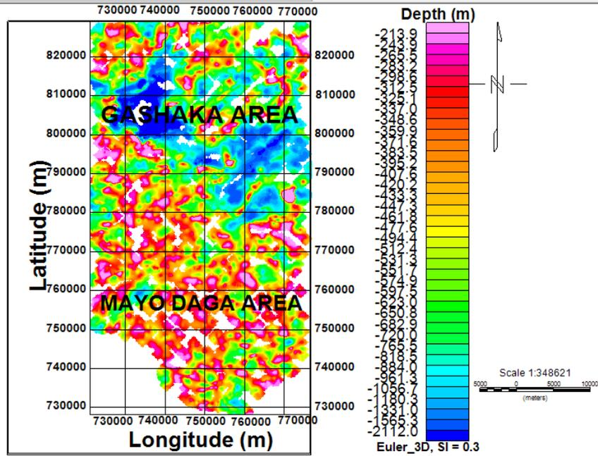
Figure 7a: Depth estimation by Euler deconvolution for structural index of 0.3.
