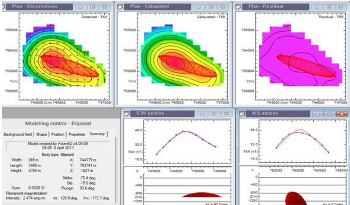
Figure 9c: Model (Ellipsoid) result of profile 3.
