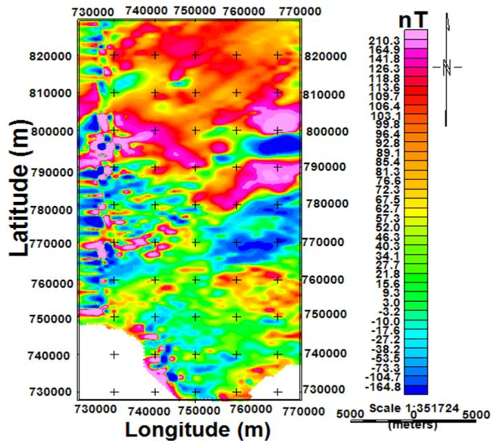
Figure 5: Upward continuation produced from residual magnetic map.
