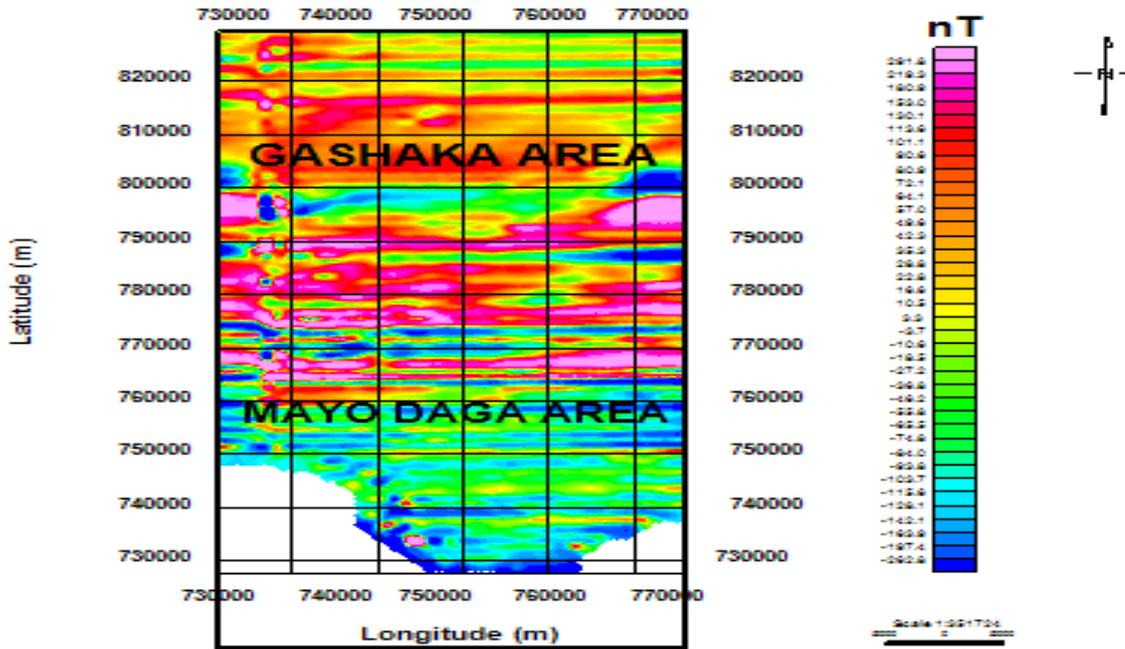
Figure 4: Reduction to Pole produced from residual magnetic map.
