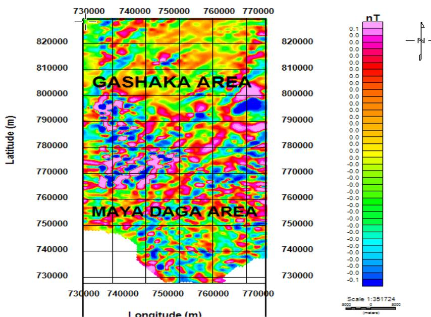
**Figure 6:** First vertical derivative produced from residual magnetic map.
