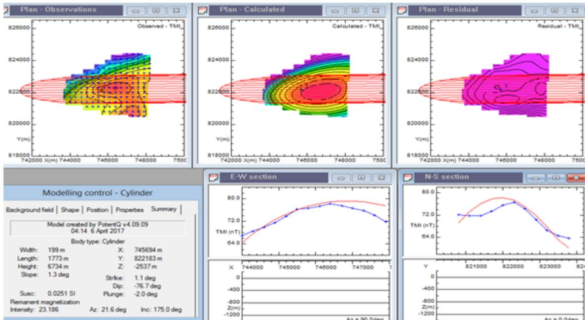
Figure 9b: Model (Cylinder) result of profile 2.
