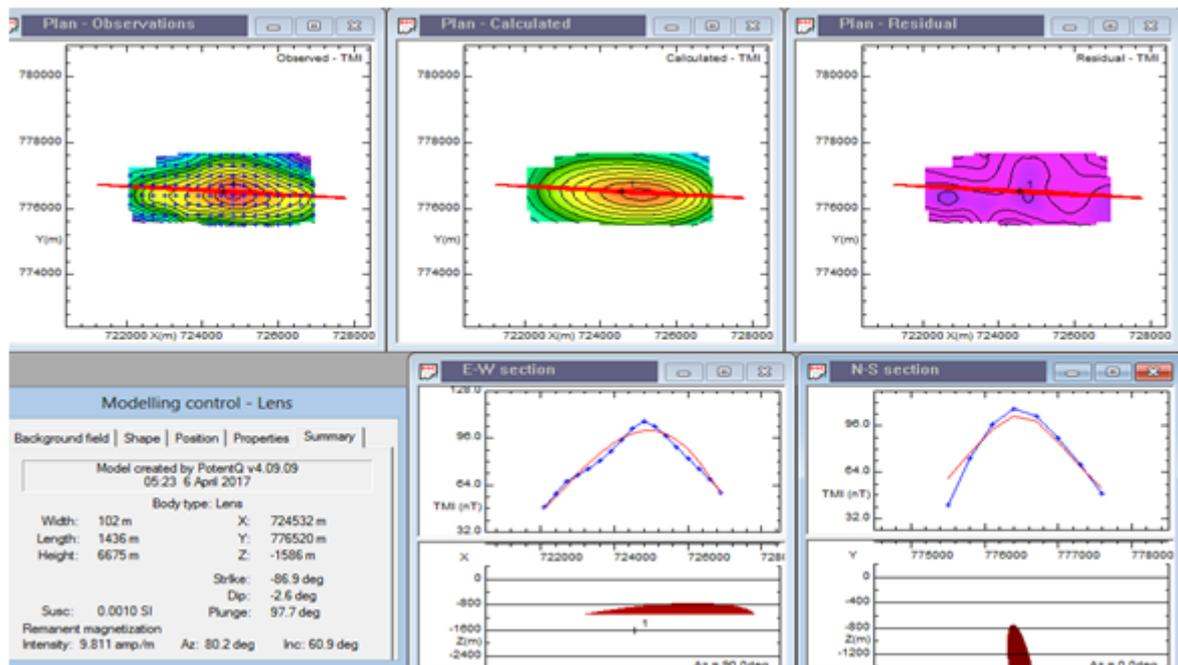
Figure 9d: Model (Lens) result of profile 4.
